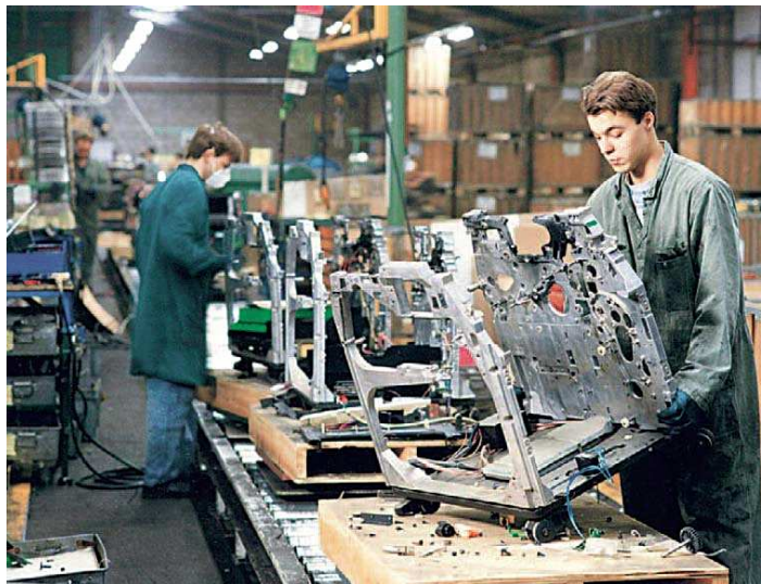
Figure 3. Disassembly line of copying machines for the reuse of parts [Steinhilper 1999].
